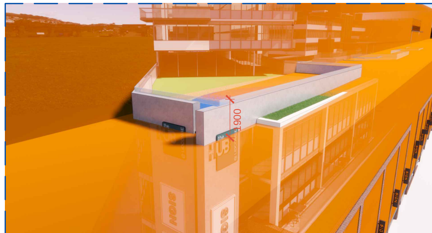
S2-PARAPET WALL AND BALUSTRADE
